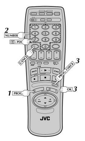
Before performing the following steps, insert a cassette with the safety tab in place. The recorder power will come on automatically.
